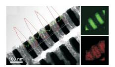
Stripped wires: Multifunctional (magnetic and optical) iron-gold barcode nanowires were electrochemically fabricated using nanoporous templates. Structural analysis by TEM elemental line scan and mapping (see images) clearly revealed the well-separated, bamboo-like nanostructures composed of Fe and Au strips.
