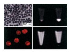
Lighting things up: Multifunctional silica nanoparticles containing a luminescent core and a paramagnetic coat are prepared, and their utility as multimodal imaging probes is demonstrated in vitro. Monocyte cells can be labeled with the hybrid nanoparticles with greater than 98% efficiency and do not experience measurable toxicity even at a high loading of 0.123 mg per 5000 cells.
